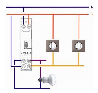
. 4 "NO" pulse operated latching relay
