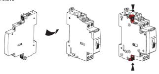
. Option of adding two auxiliaries per pulse operated latching relay, either two auxiliary contacts or one auxiliary contact and one centralised control auxiliary
